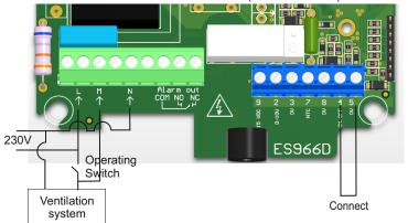
Or a potential free contact is inserted between terminal 4 and 5, as shown
