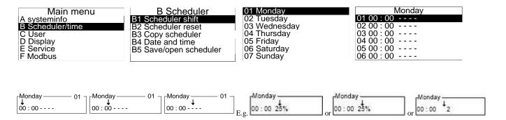
Set time for the requested shift and press "enter" & Then set required level (OFF/ON, 0-100%, Step 1-4)
