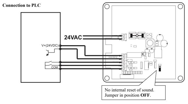
In this situation the visual and audible signals are controlled by the PLC. It is not possible to mute the sound internally, but the PLC will receive a signal when the sound mute button is pressed.
