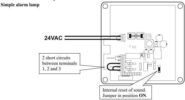
As soon as 24VAC is connected, the visual and audible alarms will be active. It is possible to deactivate the audible alarm by activating the sound mute button. To reactivate the audible alarm, disconnect and reconnect 24VAC.
