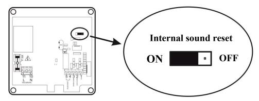
When the jumper is placed in position **ON**, it is possible to mute the audible alarm by pressing the sound mute button. It is possible to reactivate the sound by removing and reactivating the sound input on terminal 3.
