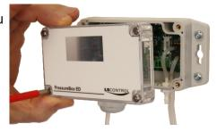
Hold down button 1 for approx. 15 sec. until display changes to show 'SCALEMAX' and the current pressure scale setting is shown.
