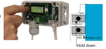
Push button 1, with each push the scale value changes in display. Stop when required scale is shown.
