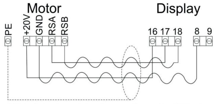
Shielded cable (max length 20m) 2 x 2x0,5mm<sup>2</sup> Twisted pair
